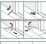
When sawing the panels make sure that the expansion gap under the door is 8mm.
