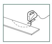
For any other cuts, you need to saw the planks. Depending on the type of saw, position your plank with the decor side face-up or face-down. Before making the actual cut, use a leftover piece to determine how the cleanest cut can be obtained (decor side face-up or face-down).
