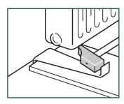
In places where it is difficult to install the planks with the tapping block (e.g.underneath radiators), you can tap them together with the pulling iron and a hammer.
