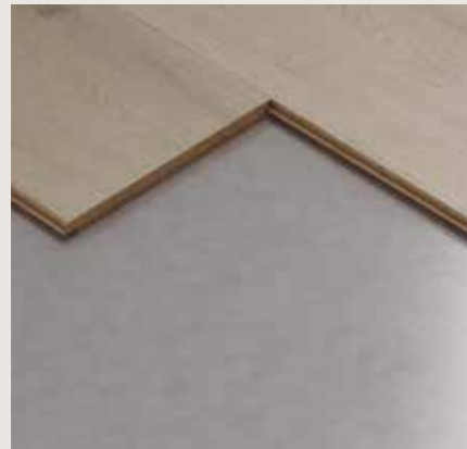
FOAM+ UNDERLAY CONCRETE SUBFLOORS Qualitative and budget-friendly underlay for rooms where there is less traffic. It has an integrated vapour barrier with an overlap and tape strip. Compatible with underfloor heating. Thickness 2 mm. 15 m 2 /roll. PGUDLFOAMPLUS15
