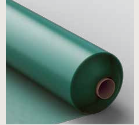
PE FILM (POLYETHYLENE) 12,5 × 2,7 m = 33,75 m 2 /roll. Protects flooring from moisture vapour rising from a mineral or concrete subfloor. Useful lifetime 50 years. Thickness: 0,2 mm. Material: Polyethylene, alkaline resistant. PGUDLSCREEN34
