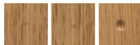
Wear layer 0,6 mm oak Wear layer 2 mm oak Solid oak
